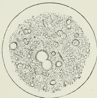
FIG. 88.—Microscopic section of chalk from Sussex. Magnified about 220 diameters.
